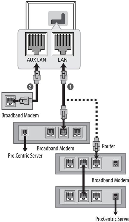
**1** Connect the **LAN** port of the Modem or Router to the **LAN** port on the TV.
