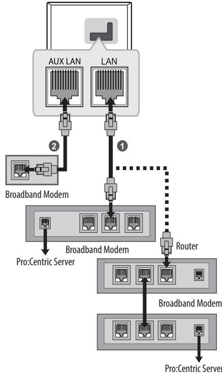
① Connect the **LAN** port of the Modem or Router to the **LAN** port on the TV.
