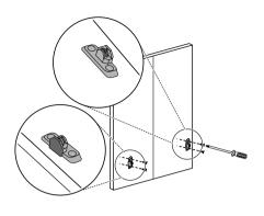
5 Attach a handle to the front of the door panel before mounting the panel on the dishwasher. Make sure to countersink the screws so the panel slides smoothly.
