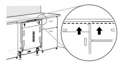
2 Measure the difference in height (X mm) between the top of the dishwasher door and the tops of the surrounding cabinet doors or drawers.
