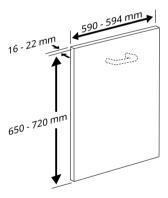
If the door panel weighs between 8 kg and 11 kg, adjust the door spring tension to make the door easier to open. See the Adjusting Door Spring Tension section.
