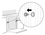
**2** Drive a wood screw (Φ 4 x 16 mm) through the mounting bracket and into the cabinet frame.
