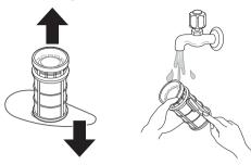
4 To replace the assembled filters, position the spray arm so the wider vee is toward the front. Fit the filters back into the filter holder and secure them by turning the inner filter clockwise until it clicks into place.
