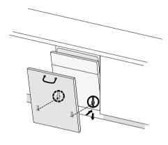
2 Remove the 2 screws from the front cover. Attach the door panel to the dishwasher door using the provided wood screws (Φ 4 x 40 mm).
