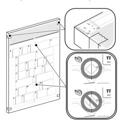
3 Use a 2 mm diameter drill bit to drill 10 mm deep pilot holes at the 10 points marked on the template.
