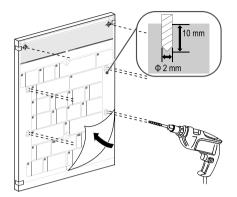
Remove the template, and attach the upper and middle panel brackets (provided) to the door panel using the provided bracket screws (Φ 4 x 14 mm).
