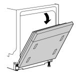
Use the door adjustment screws (Φ 4 x 34 mm) provided to adjust the door spring tension at the bottom of the dishwasher.
