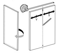
Align the top and centre line on the installation template with the top and centre line of the door panel. Securely tape the installation template to the back of the door panel.
