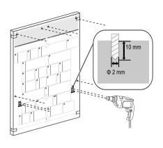
4 Remove the template, and attach the panel brackets (provided) to the door panel using the provided bracket screws (Φ 4.5 x 12 mm).
