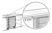
3 Using the measurement from step 2, make a mark (X mm) up from the bottom of both rulers at the top of the provided installation template.
