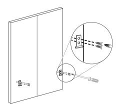
**5** Attach a handle to the front of the door panel before mounting the panel on the dishwasher.
