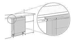
Using the measurement from step 2, make a mark (X mm) up from the bottom of both rulers at the top of the provided installation template. Draw a line between the marks and trim off the top of the template at the line.
