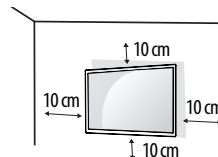
If you intend to mount the TV to a wall, attach Wall mounting interface (optional parts) to the back of the TV. When you install the TV using the wall mounting interface (optional parts), attach it carefully so it will not drop.
