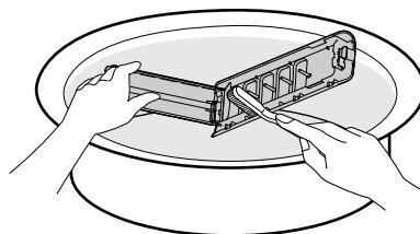
**4** Close the lid and then insert the lower part of the filter into the wash drum. Press the top of the filter until you hear a **click sound**.
