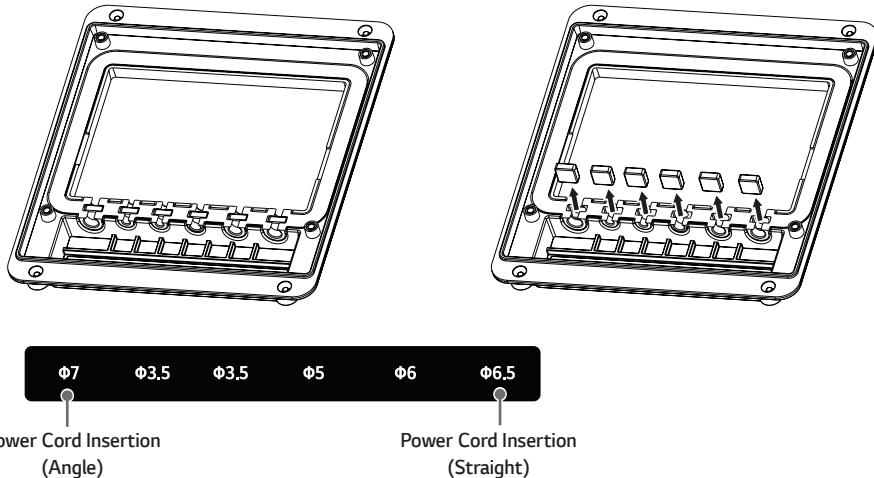
Remove the square rubbers before connecting the cables.
