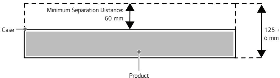
**When Drilling the Inlet and Outlet on the Side of the Case**
