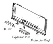
• Only remove the protection vinyl when using a side screw hole.
