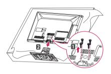
3 Push the supplied protection cover into the opening at the bottom of the TV until it locks in place.
