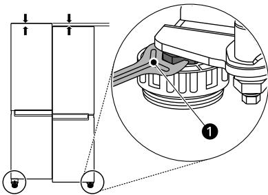
2 Use the spanner ② to adjust the height by turning the adjustment hinge pin to the left or to the right.
