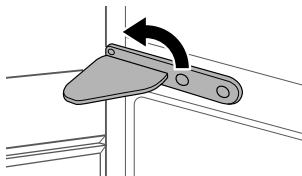
**3** Remove the door by lifting it off the lower hinge pin.
