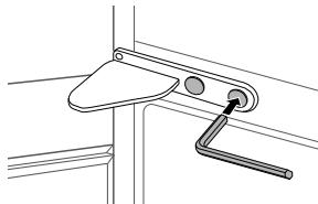
**2** Twist the hinge to raise the pivoting end so that the door can be lifted off. Lift the door off the lower hinge pin and remove it.
