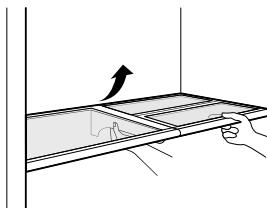
2 Tilt the shelf at an angle and pull it out.
