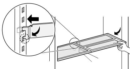
3 To assemble, tilt the front of the shelf up and guide the shelf hooks into the slots at a desired height.
