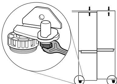
3 Use the spanner ① to fasten the keeper nut by turning it to the right.
