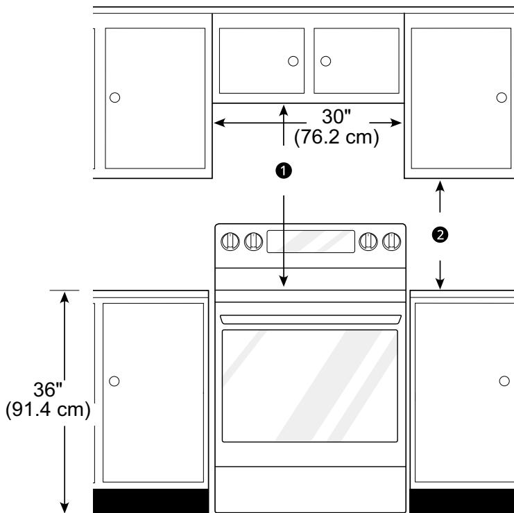
① 30" (76.2 cm) minimum clearance between the top of the cooking surface and the bottom of an unprotected wood or metal cabinet; or 24" (60.9 cm) minimum when bottom of wood or metal cabinet is protected by not less than 1/4" (0.64 cm) flame retardant millboard covered with not less than no. 28 MSG sheet steel, 0.015" (0.381 mm) stainless steel, 0.024" (0.610 mm) aluminum or 0.020" (0.508 mm) copper.
