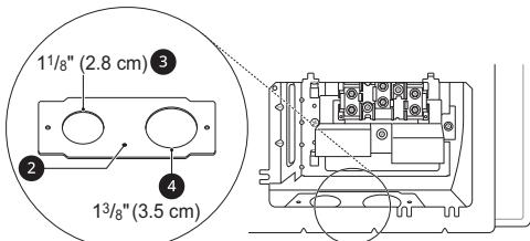
For power cord ⑤ installations, hook the strain relief over the 1 3/8 in. (3.5 cm) power cord hole located below the rear of the oven. Insert the power cord through the strain relief and tighten it.
