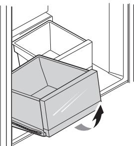
2 With the drawer fully extended, lift up the front and pull the drawer out to remove it.
