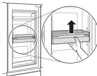
**2** To lower the moving basket, press up to release the levers at the side of the basket and lower the basket until it clicks into place.
