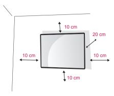
Install the monitor at least 10 cm away from the wall and leave about 10 cm of space at each side of the monitor to ensure sufficient ventilation.
