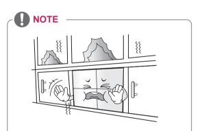
Do not install the product in a place with no ventilation (e.g., on a bookshelf or in a closet) or on a carpet or cushion. If there is no other option but to mount the product on the wall, make sure that sufficient ventilation is provided before installation.
