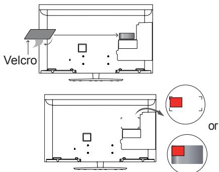
\* Attach the RF dongle aligning with the upper left corner bracket.
