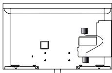
\* If the RF dongle for the wireless media box is attached, attach the RF dongle for the Magic Motion remote control on the upper right of the back of the TV.
