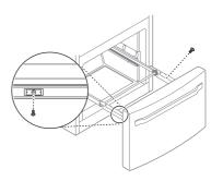
4 Insert the drawer into the frame, and push the drawer back until it clicks into place.
