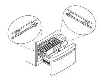
5 Replace the ice bin in the drawer. Insert the Durabase basket in the rail assembly.
