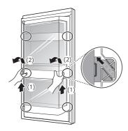
2 To replace the Door-in-Door case, line up the tabs on the Door-In-Door case with the slots on the door and push down until it snaps into place.
