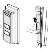
**2** Lift up and remove the baskets from the door in door casing.
