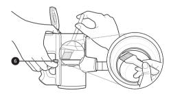
**8** Turn the product body over again and shake it while pressing down the lever to remove the dust.
