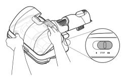
2 Place the mop nozzle on the floor, turn on the power, and let it run for about 1 minute.
