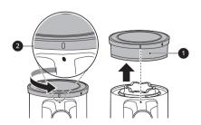
**3** Grip the exhaust filter cover **3** and the exhaust filter **1** using both hands and rotate the exhaust filter cover while pressing the **PUSH**
