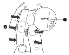
Push and insert the exhaust filter cover into the exhaust filter and rotate it to reassemble it and prevent it from falling out.
