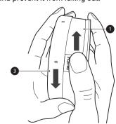
9 Insert the dried pre-filter and rotate the exhaust filter to the locked position **6** to reassemble it on the product body.
