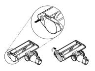
3 Pull the brush cover forward and pull the main brush out.
