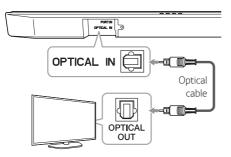
Select the input source to OPTICAL by pressing F button on the remote control or unit repeatedly.
