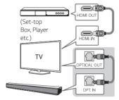
2 Set the input source by pressing **OPTICAL** on the remote control or pressing **F** repeatedly.
