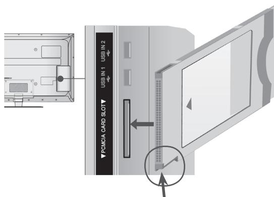
Check this point as shown and insert the CI Module.
