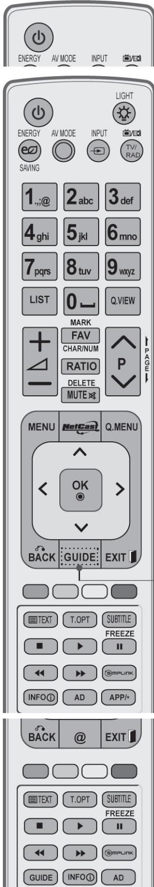
**⏻ (POWER)** Switches the TV on from standby or off to standby.
