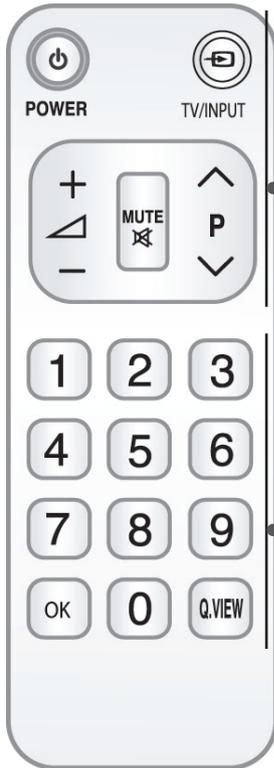
**⏻ (POWER)** Switches the TV on from standby or off to standby.
