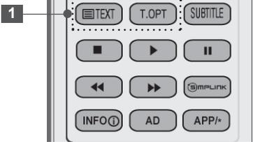
**1** **TELETEXT BUTTONS** These buttons are used for teletext.
