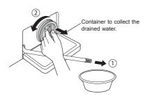
3 Remove any extraneous matter from the pump filter.
