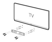
5. Hang the main unit onto the bracket as shown below.
