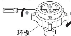
**2 如果水龙头过大而与接头不匹配，请拆下导向板。**
