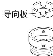
**3 将接头往上推至水龙头末端，从而使橡胶密封圈形成水密连接。拧紧四颗固定螺丝和接头环板。**
