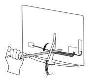
Do not use a sharp object when you detached the cable cover. This could damage the cable or the cabinet. It may also cause personal harm. (Depending on model)  When installing the wall mounting bracket, it is recommended to cover the stand hole using tape, in order to prevent the influx of dust and insects. (Depending on model)
