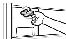
5 Lift and remove the ice storage bin slightly.
