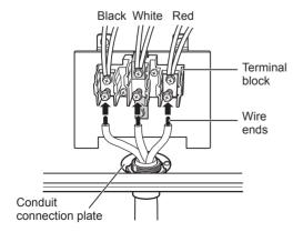
If screws are not tightened securely, it can result in electrical spark and severe personal injury or death.
