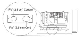
Remove the conduit connection plate
