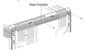
2 Attach the rear bracket and filler assembly as shown, using the three screws removed in step 1.
