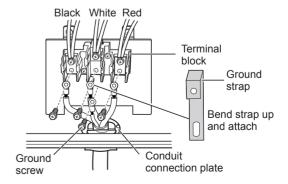
If screws are not tightened securely, it can result in electrical spark and severe personal injury or death.
