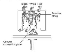
If screws are not tightened securely, it can result in electrical spark and severe personal injury or death.
