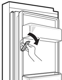
2 To remove the in-door ice bin, grip the front handle, lift up slightly while holding both the top and bottom parts (1), and slowly pull out the bin as shown (2).
