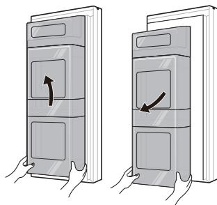
2 Lift and remove the bottom of the dairy basket from the whole case.
