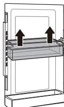
4 Lift and remove the moving basket from the case after remove the screws from each of the side rails.
