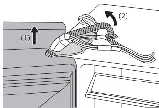
Lift the upper hinge fixed between the appliance and the appliance door and then remove it.
