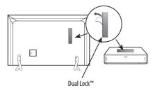
2 Attach the set-top box to the TV by pressing the Velcro strips together.
