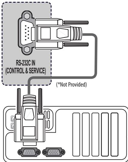
**Type of Connector : D-Sub 9-Pin Male**
