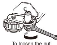
2 Adjust the difference in the height of the appliance door by rotating the adjustment hinge pin clockwise or counterclockwise with an 8 mm spanner.
