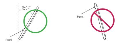
When installing the monitor, it may be tilted upward at an angle of up to 45 degrees.
