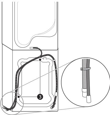
band clamp ① to keep the washer hose in place.
