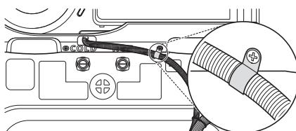
6 Use the provided tie strap ③ to secure the 2 drain hoses in place.
