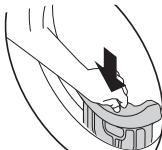
regularly to remove any build-up of lime scale on the surface of the sensor.
