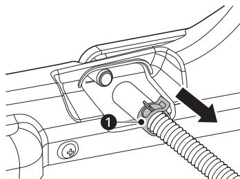
3 Connect the drain hose of the dryer and secure the hose clamp.
