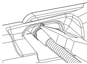
4 Loosen the screw ② on the stack bracket.
