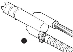
3 Use the band clamp ② on the short drain hose (included) to attach it to the bottom opening of the drain hose connector.
