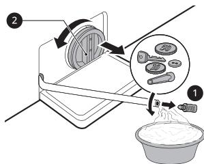
4 After cleaning the drain pump filter, carefully reinsert the filter and screw the drain cap back in clockwise carefully to avoid cross threading and leakage. Reinsert the plug back into the drain tube and place the tube into its holder.
