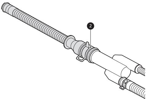
4 Connect securely the short drain hose to a floor gully or a standpipe.
