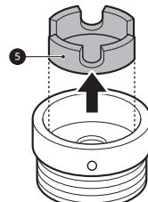
3 Push the adapter onto the end of the tap so that the rubber seal is connected to be watertight. Tighten the 4 fixing screws and the adapter ring plate.
