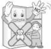
**Do not lean on the doors, Hinges may deregulate themselves, causing air leak and performance deterioration**
