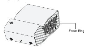
To bring images into focus, move the Focus Ring slowly up or down, concentrating on the upper central part of the screen. Optimal focus is reached when the left and right sides of the screen appear balanced.
