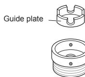
3 Push the adapter onto the end of the tap so that the rubber seal forms a watertight connection. Tighten the four fixing screws.
