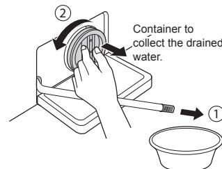
3 Remove any extraneous matter from the pump filter.
