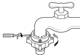
**4** Pull the connector latch plate down, push the supply hose onto the adapter, and release the connector latch plate. Make sure the adapter locks into place.
