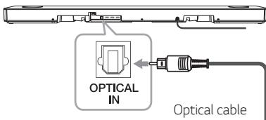
1. Connect the OPTICAL IN jack on the back of the unit to optical out jack of your external device.
