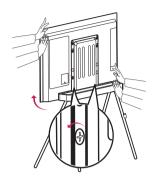
Loosen the screw halfway by using a Phillips screwdriver, adjust the height on both sides of the TV as illustrated, and tighten the screw.
