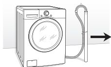
Connecting the drain line
