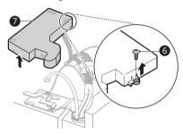
3 Remove the cover and pull out the tube **3**. Disconnect all wire harnesses **9**. Unscrew the ground wire **0**.
