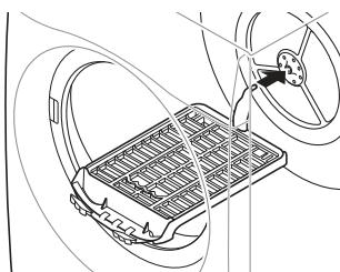
3 Place the dryer rack on the structure above the lint filter and press it to complete assembly.
