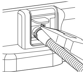
3 Screw in the band to secure the drain hose of the dryer onto the stacking bracket.
