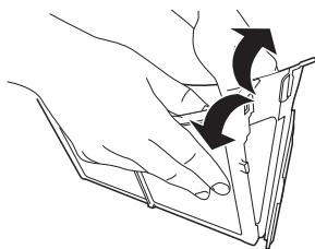
5 Clean the residual lint filter by hand or using a vacuum cleaner.
