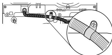
4 Use the provided tie strap ② to secure the 2 drain hoses in place.
