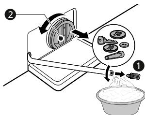
**4** After cleaning the drain pump filter, carefully reinsert the filter and screw the drain cap back in clockwise carefully to avoid cross threading and leakage. Reinsert the plug back into the drain tube and place the tube into its holder.
