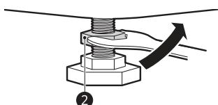
**4** Check if all lock nuts at the bottom of the appliance are secured properly.
