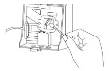
After inserting the rubber cover 3, assemble the PM1.0 sensor cover 2.
