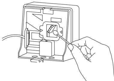
Tighten the rubber cap, close the PM1.0 sensor case, and assemble the PM1.0 Sensor corner cover to its original position.
