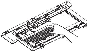
4. Wash the filter after checking the washing method in 'Filter Information'.
