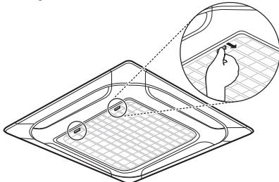
2. Remove PM1.0 filter by pressing the fixing hook.
