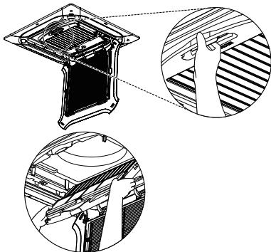
3. Remove the photocatalyst Deodorization filter by pulling upward.
