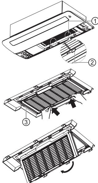
3. As shown in the figure, pull on the handle and remove the deodorization filter.
