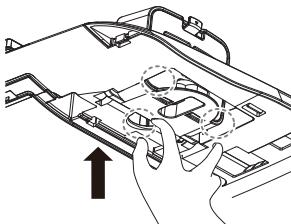
2. Open the front panel and lower the PM1.0 Sensor case as shown in the figure below.
