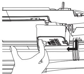
4. Open the PM1.0 sensor cover on the side of the case.
