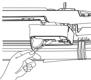
6. Close the PM1.0 Sensor case cover, then install the PM1.0 Sensor case in its original position.
