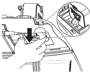
3. Once the PM1.0 Sensor case is lowered all the way, turn the PM1.0 Sensor case to secure it as shown in the figure below.
