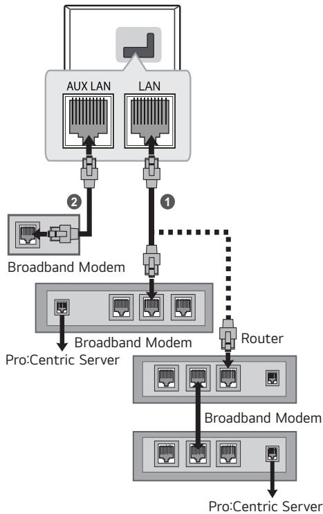
① Connect the **LAN** port of the Modem or Router to the **LAN** port on the TV.
