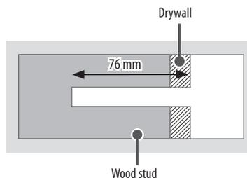
Use the  $\varnothing$  4 mm drill bit for wood to drill holes with the depth of 76 mm. (Clean the drilled hole.)
