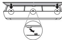
8 Check the side of the front cover for correct assembly of the air filter.
