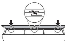
7 Push down hooks to assemble the air filter.
