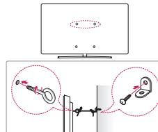
1 Insert and tighten the eye-bolts, or TV brackets and bolts on the back of the TV.
