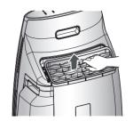
2. Use the cleaning brush and cleaner inlet to remove the dust on the safety blocking net.
