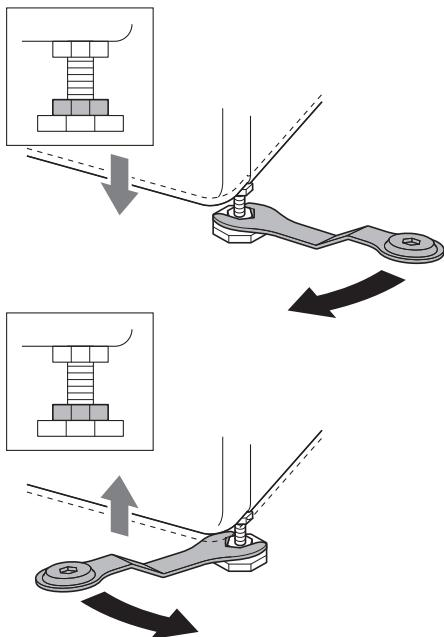
**3** Secure the levelling feet with the lock nuts ② by turning anti-clockwise against the bottom of the appliance.
