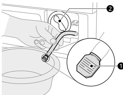
**4** Clean the pump filter and opening with a brush.
