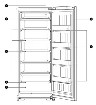
1 Temperature Control (on back wall of compartment)
