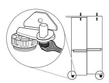
Open the door and use the spanner 1 to loosen the keeper nut by turning it to the left.
